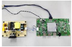
Step.10 Remove connecter cable and separate main board and power board
