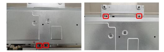
Step.7 pull out 2 Pcs connectors and remove main-shielding from LCM
