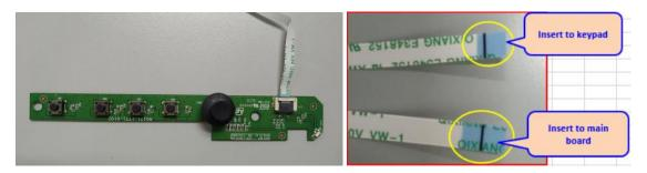
Step15. Fix keypad on rear cover by screws, then use yellow tape to tape FFC. Insert FFC to main board.
