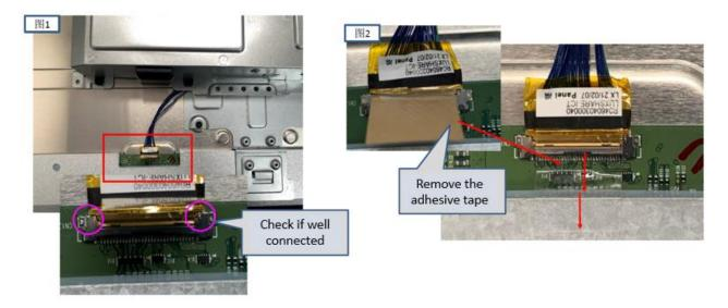
Step8. Insert 6P backlight cable to panel
