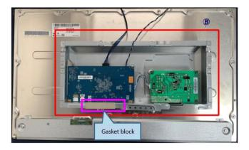
Step7. Insert 30pin FFC to panel
