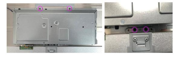
Step10. Assembly middle frame with panel and fix by screws (in red circle).
