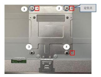
Step6. Tape gasket block on shielding
