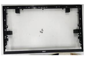
Step.12 Use screwdriver unscrew 4pcs screws and separate shielding holder from the LCM
