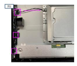
Step12. Assembly speaker on middle frame, and assembly speaker cable on main board. (red and white cable is on left side, yellow and black is on right side.)
