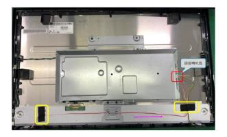
Step14. Fix navi key on keypad, and insert 8pin FFC to connecter.
