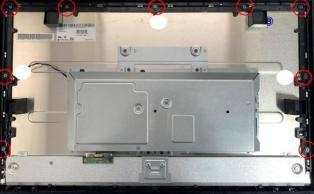
Step11. Tape 1pcs CR sponge on the left side, and fix the backlight LVDS into the hook of mid frame.
