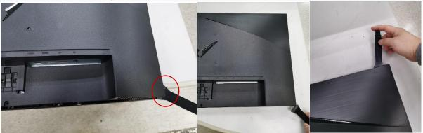
Step 4. Pull up the Rear Cover and pull out 2 pcs connecters
