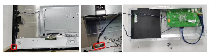
Step.8 Separate mylar and move wires from shielding's hook
