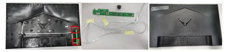
Step.14 Use screwdriver unscrew the screw and separate base & neck assembly
