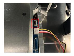
Step14. Assembly rear cover, and push around the surrounding to assembly well.
