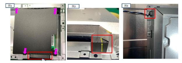
Step5. Fix the bracket on panel by 4 screws.
