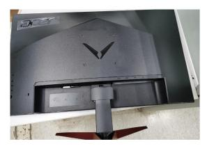
Step.2 Unscrew four screws using a screwdriver
